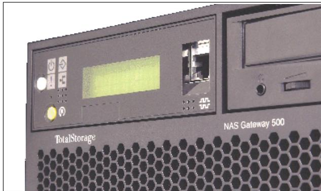
Figure 7-2 NAS Gateway 500 LCD operator panel
